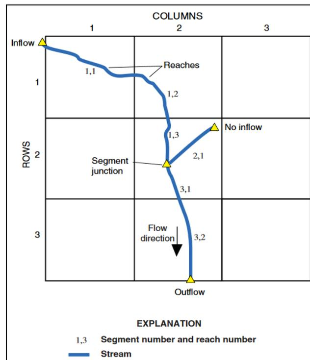
Figure 6 Illustration of stream segment and reach numbering<sup>5</sup>
