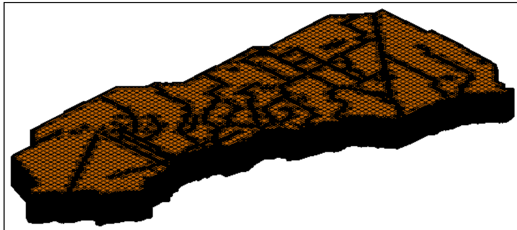
Figure 10 2D UGrid extruded to a 3D UGrid
