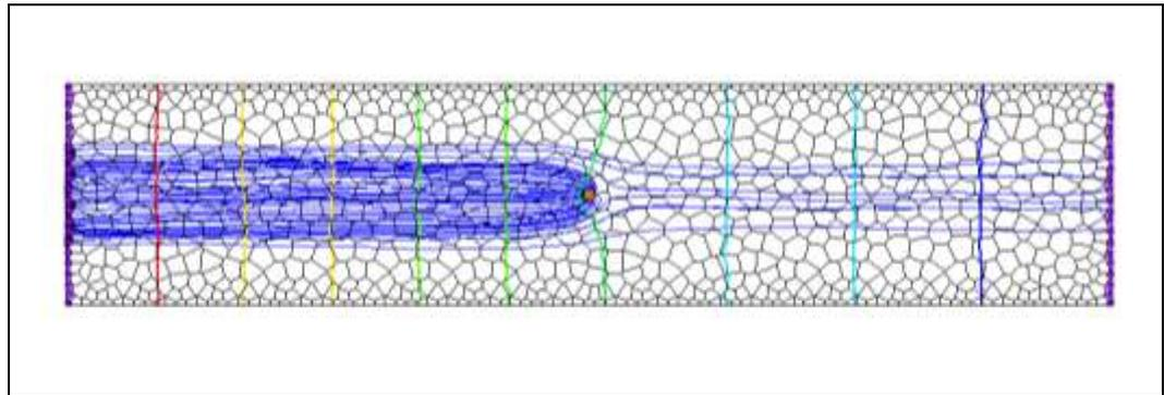
Figure 10 Pathline solution showing pathlines tracking backward from the well.
