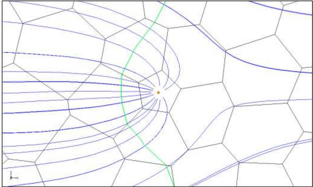
Figure 11 Forward tracking pathlines around the well.
