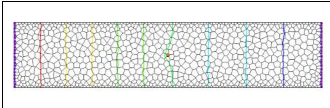
Figure 1 Nested grid example included with MODFLOW-USG.
